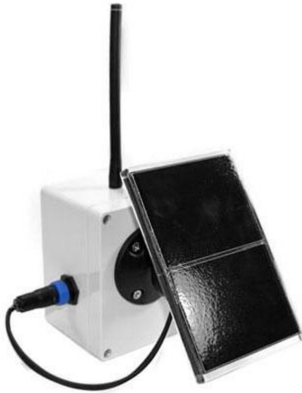
Figure 14, A base station for collecting data from a remote download GPS tag
